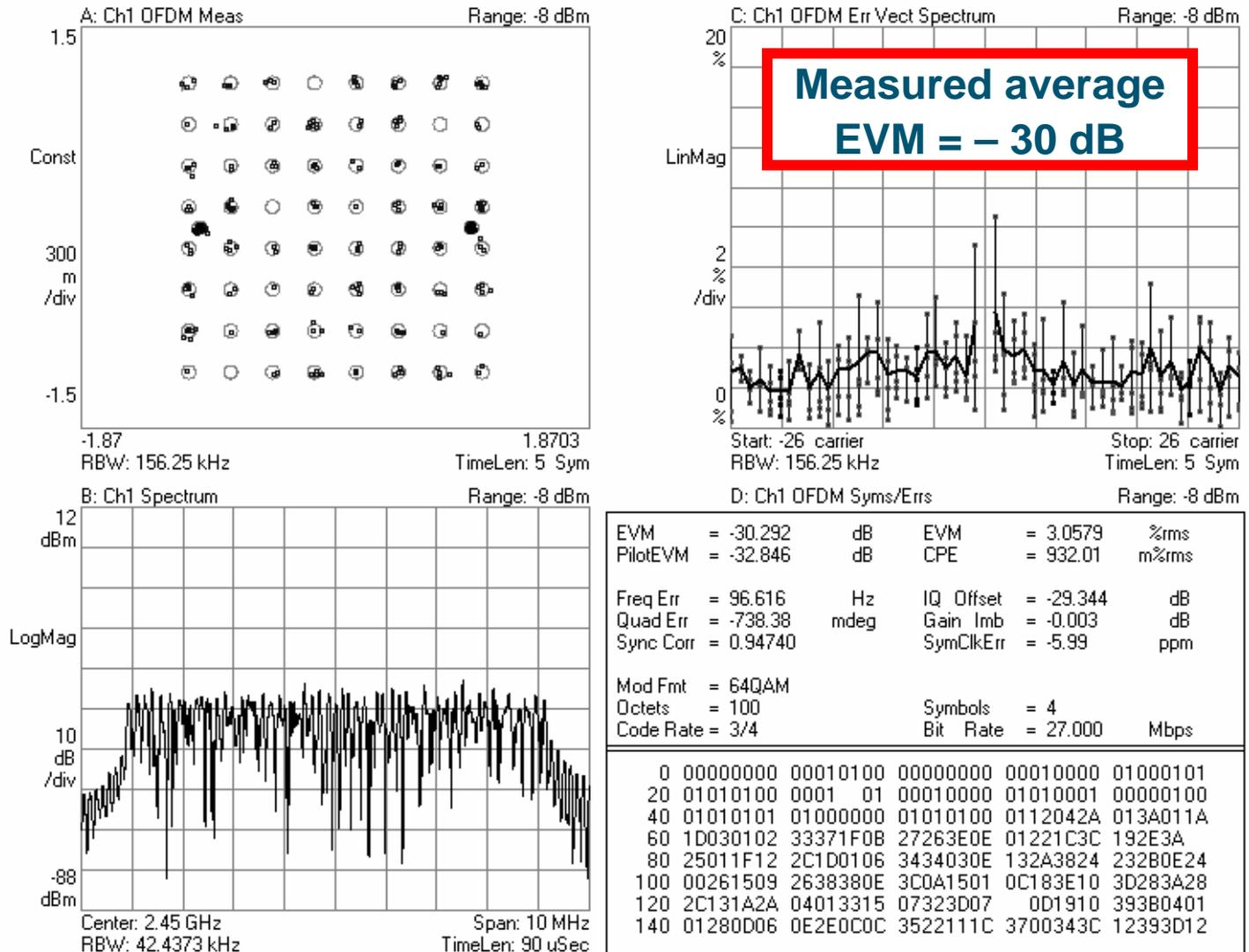
■ 1/f noise degrades the EVM near the carrier frequency
