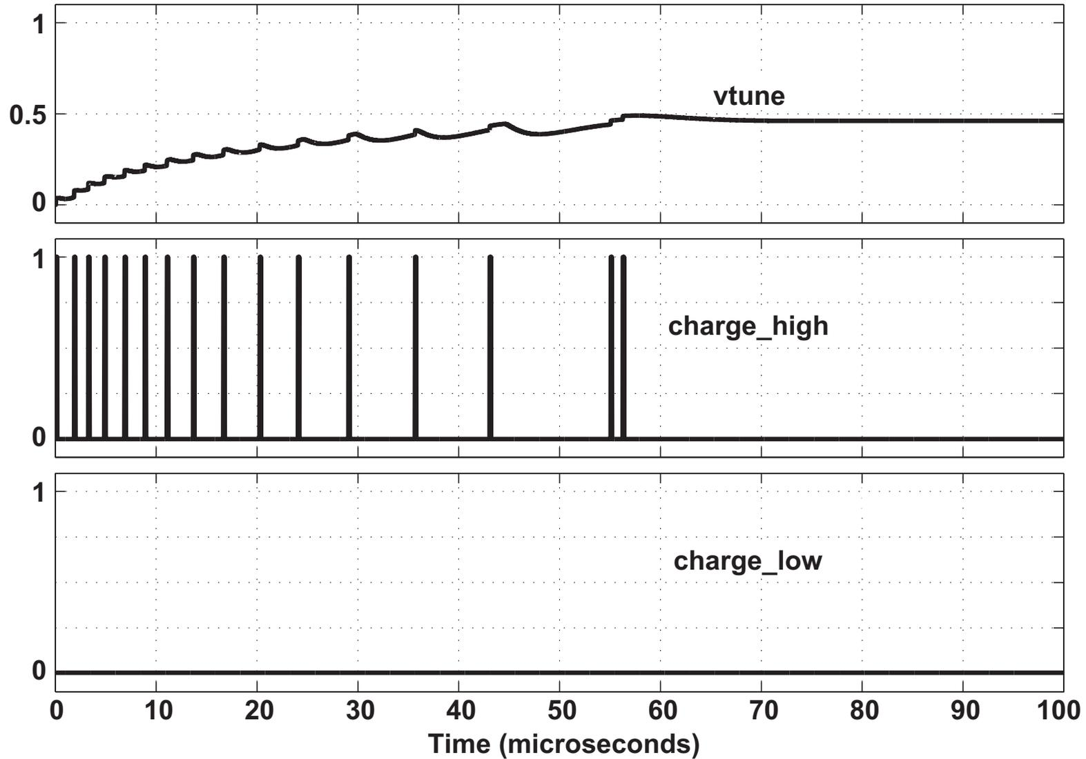
**Switched capacitor technique allows relatively fast frequency locking**
