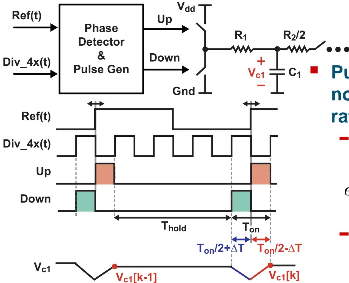
**Pulse width modulation nonlinearity is reduced as ratio  $\Delta T/(R_1 C_1)$  is reduced**
