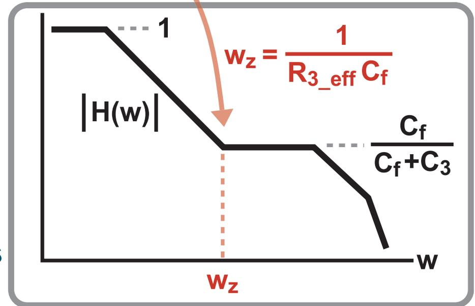
**Example: Proper choice of  $T_{on}$  and  $T_{period}$  allows  $R_{3\_eff} = 16$  MegaOhms to be achieved with  $R_3 = 500$  kOhms!**
