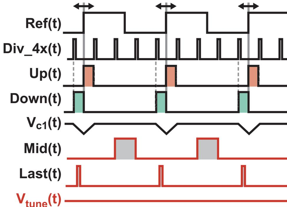
**Ripple from Up/Down pulses blocked before reaching VCO**
