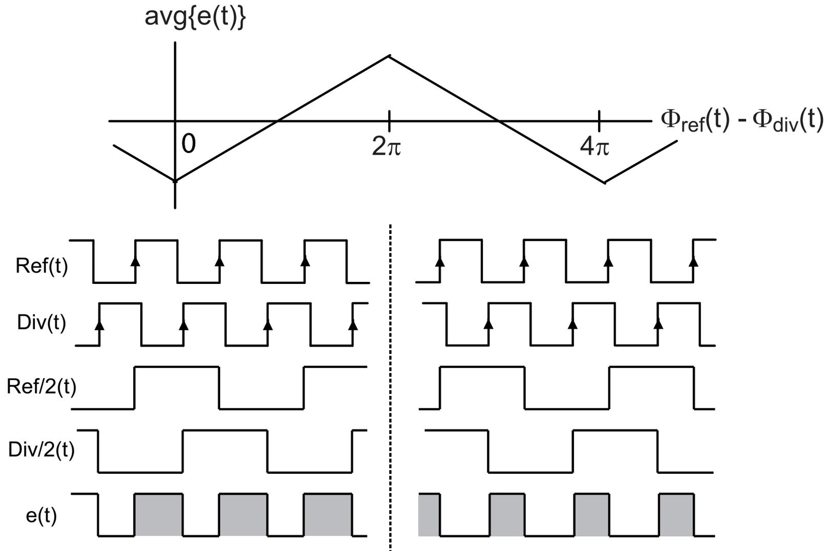
**Gain flips in sign according to phase error region of phase detector**
