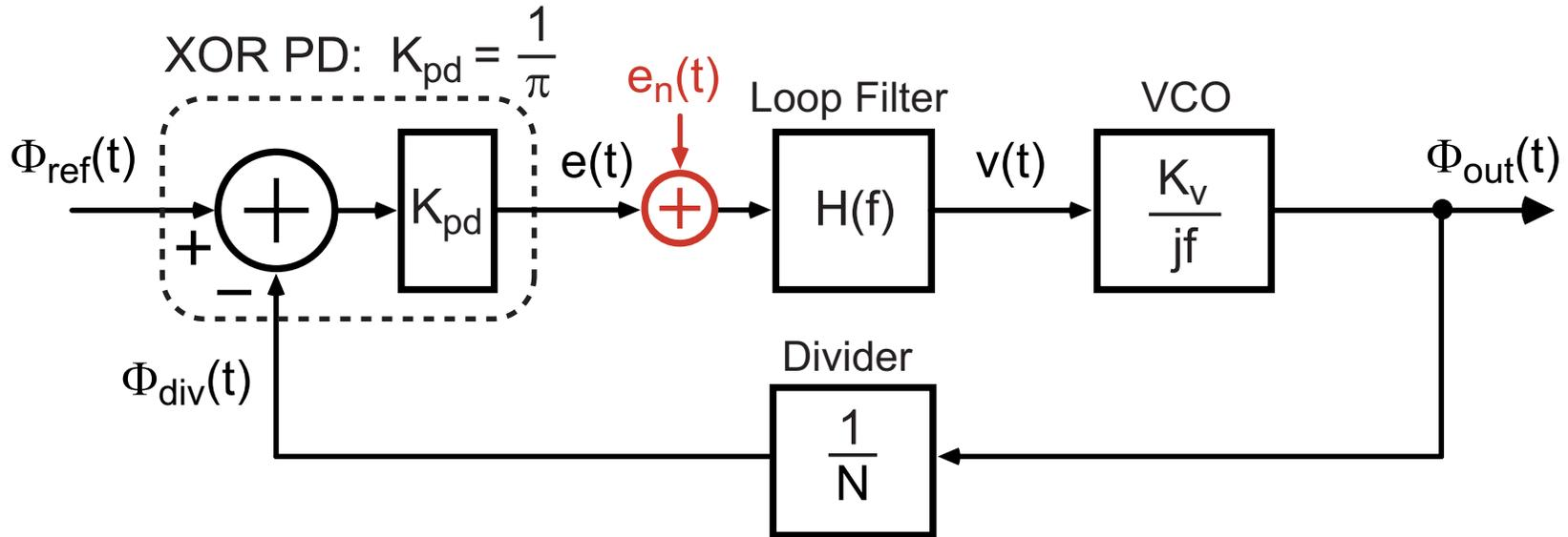
$$\begin{aligned} \frac{\Phi_{out}}{e_n} &= \frac{H(f)K_v/(jf)}{1 + (K_{pd}/N)H(f)K_v/(jf)} \\ &= \frac{N}{K_{pd}} \frac{(K_{pd}/N)H(f)K_v/(jf)}{1 + (K_{pd}/N)H(f)K_v/(jf)} \\ &= \frac{N}{K_{pd}} \frac{A(f)}{1 + A(f)} = \boxed{\frac{N}{K_{pd}} G(f)} \end{aligned}$$
