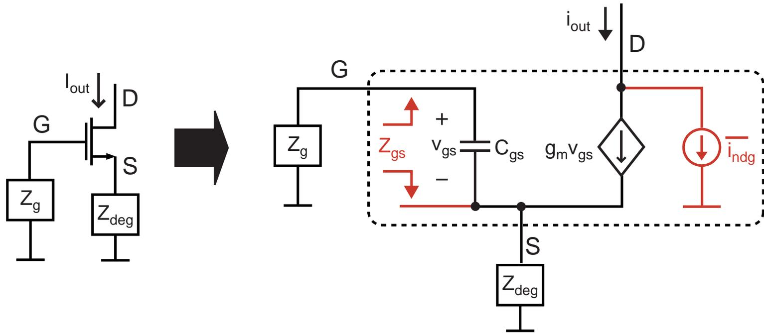
$$\frac{\overline{i_{ndg}^2}}{\Delta f} = \frac{\overline{i_{nd}^2}}{\Delta f} \left( |\eta|^2 + 2 \operatorname{Re} \{ c \chi_d \eta^* Z_{gsw} \} + \chi_d^2 |Z_{gsw}|^2 \right)$$
