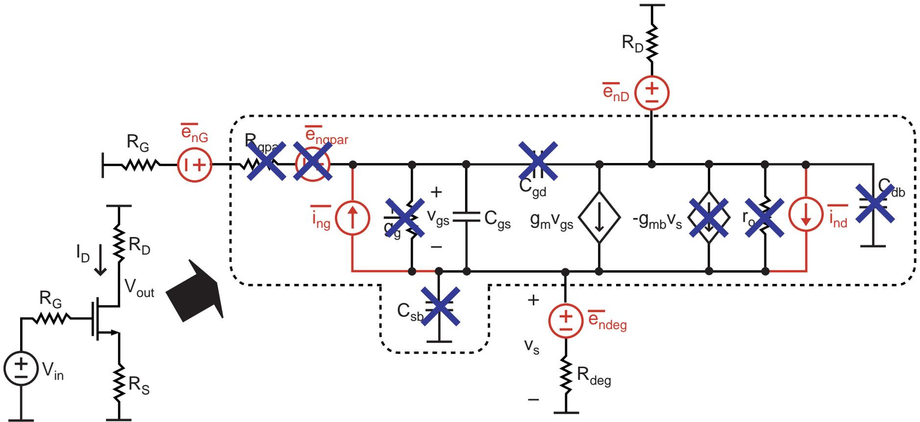
$R_{gpar}, \overline{e_{ngpar}}$  : can make negligible with proper layout
