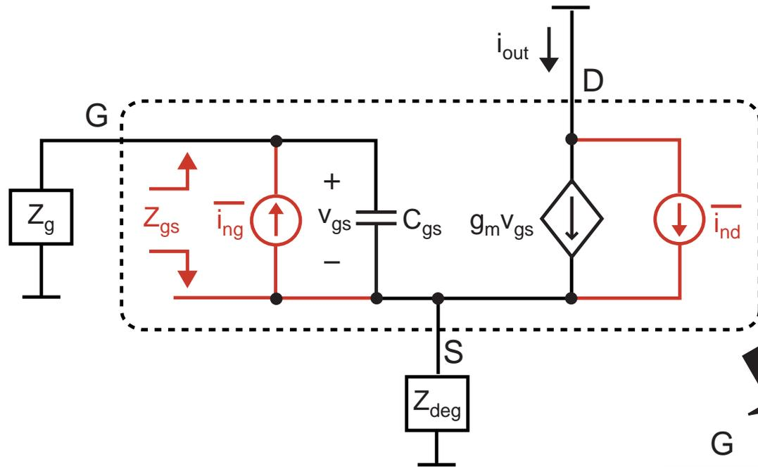
$$i_{out} = g_m Z_{gs} \overline{i_{ing}} + \eta \overline{i_{nd}}$$
