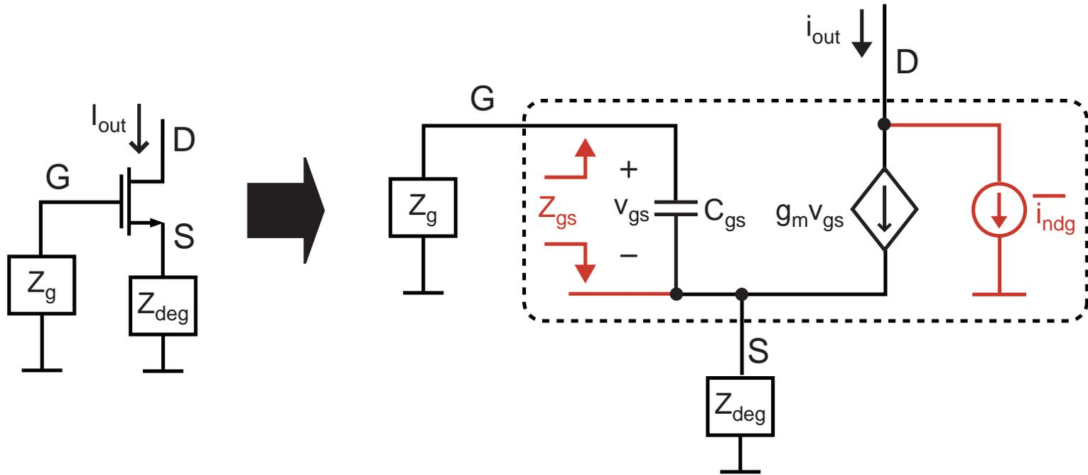
$$i_{out} = \overline{i_{ndg}} = \eta \overline{i_{nd}} + g_m Z_{gs} \overline{i_{ng}}$$
