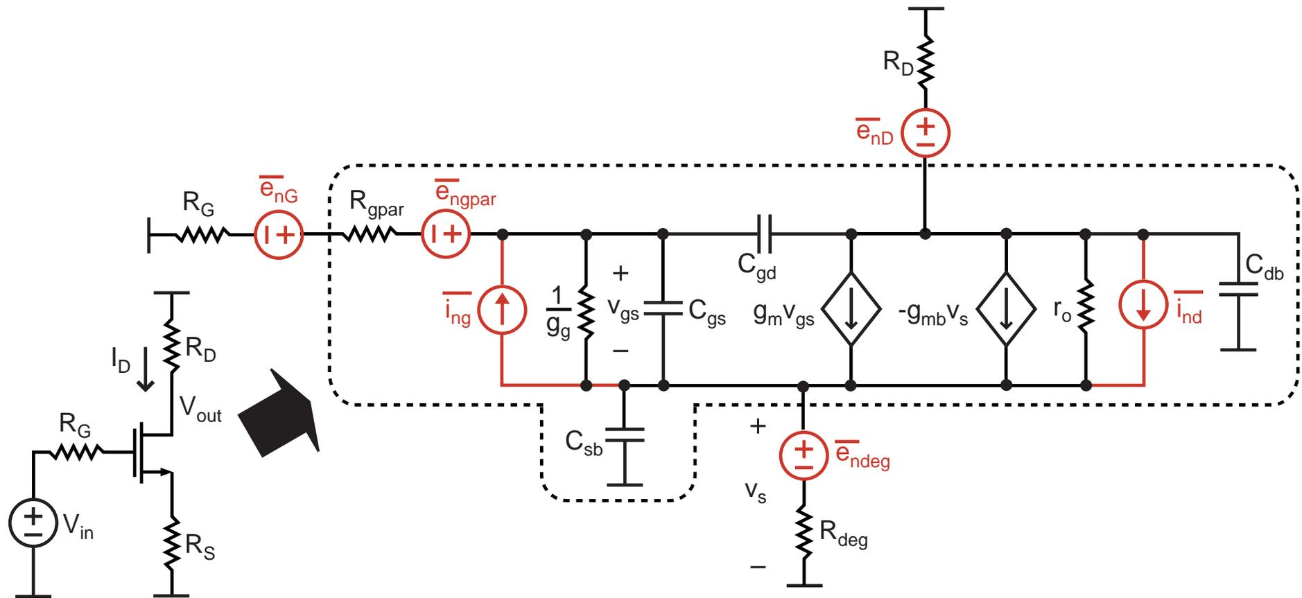
$\overline{e_{nG}}$ ,  $\overline{e_{nD}}$ ,  $\overline{e_{ndeg}}$  : noise sources of external resistors
