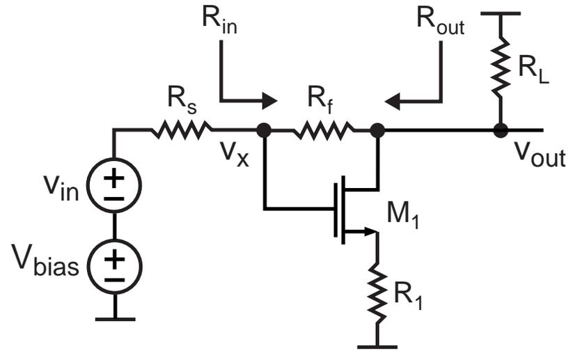
Note:  $A_v \approx -\frac{R_L}{R_1}$  for  $R_f \gg R_L$ ,  $R_f \gg R_E$ ,  $R_1 \gg 1/g_m$
