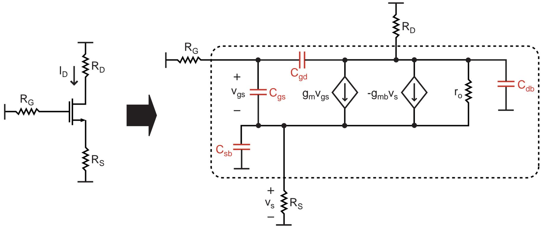
$$C_{gs} = C_{gc} + C_{ov} = \frac{2}{3} C_{ox} W(L-2L_D) + C_{ov}$$
