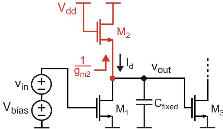
$$C_{\text{tot}} = C_{\text{db1}} + C_{\text{sb2}} + C_{\text{gs2}} + C_{\text{gs3}} + KC_{\text{ov3}} + C_{\text{fixed}}$$
