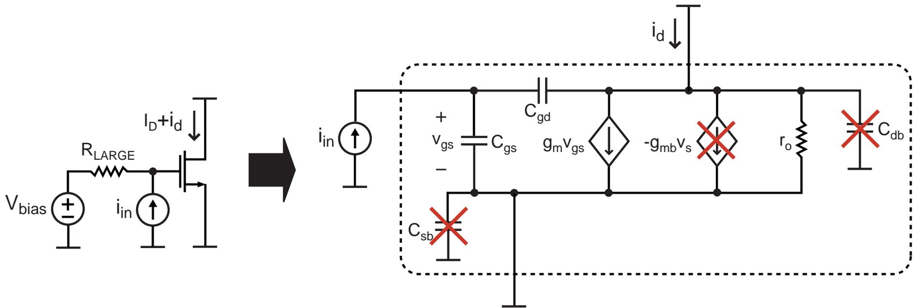
$$i_d = g_m v_{gs} = g_m \left( \frac{1}{s(C_{gs} + C_{gd})} \right) i_{in}$$
