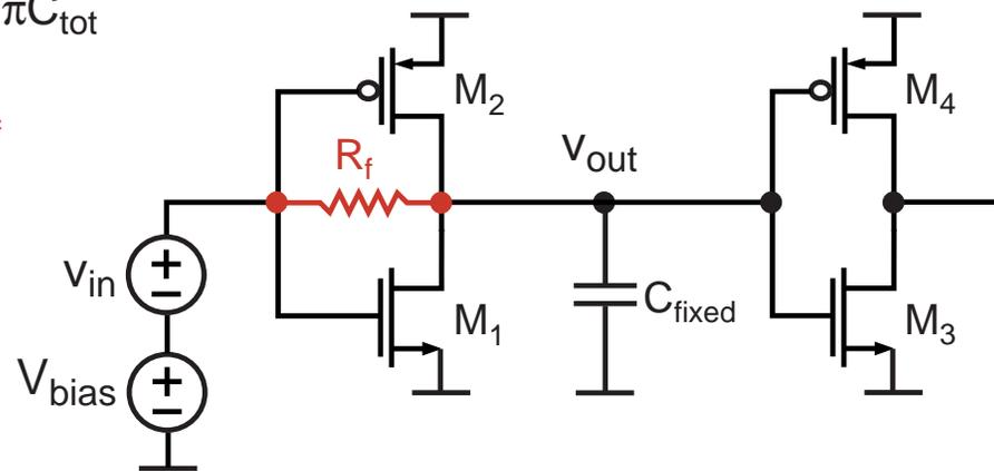
$$C_{tot} = C_{db1} + C_{db2} + C_{gs3} + C_{gs4} + K(C_{ov3} + C_{ov4}) + C_{Rf}/2 + C_{fixed}$$
