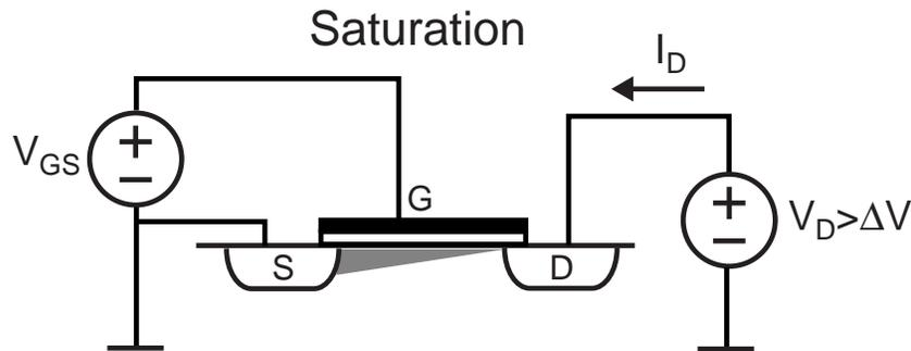
$$I_D = \frac{1}{2} \mu_n C_{ox} \frac{W}{L} (V_{GS} - V_T)^2 (1 + \lambda V_{DS})$$
