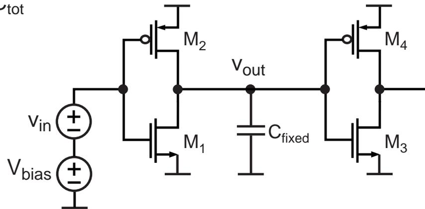
$$C_{tot} = C_{db1} + C_{db2} + C_{gs3} + C_{gs4} + K(C_{ov3} + C_{ov4}) + C_{fixed}$$
