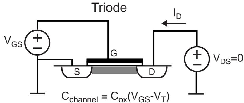
$$I_D = \mu_n C_{ox} \frac{W}{L} (V_{GS} - V_T - V_{DS}/2) V_{DS}$$
