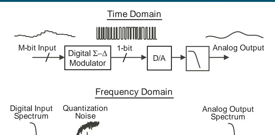
Sigma-Delta dithers in a manner such that resulting quantization noise is "shaped" to high frequencies
