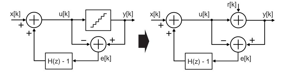
Calculate using Z-transform of signals in linearized model
