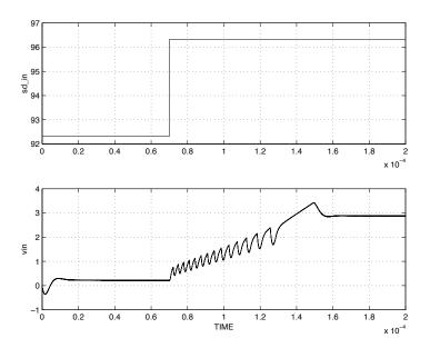
Figure 4.4 Synthesizer response to a step input — top plot: input to sd\_modulator, bottom plot: closed loop response of VCO input voltage.
