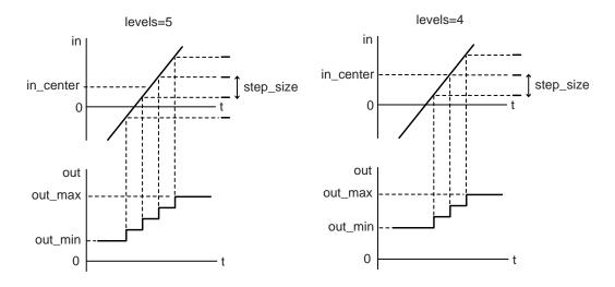
Figure 7.1 Illustration of behavior of Quantizer class in relation to parameter settings.
