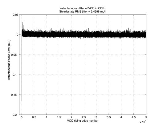
Figure A.10 Simulation plot for CDR (bang-bang phase detector).
