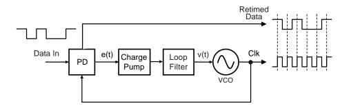
Figure A.6 A PLL-based clock and data recovery circuit.
