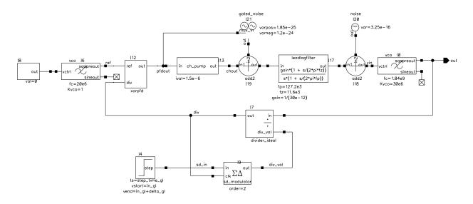
Figure 4.1 Sue2 schematic of  $\Sigma$ - $\Delta$  frequency synthesizer.
