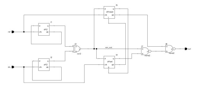
Figure 4.2 Sue2 schematic of XOR-based phase/frequency detector.
