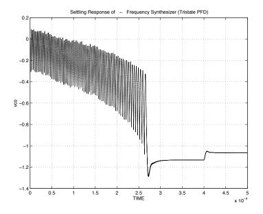
Figure A.5 Simulation plot for  $\Sigma$ - $\Delta$  synthesizer (Tristate PFD).
