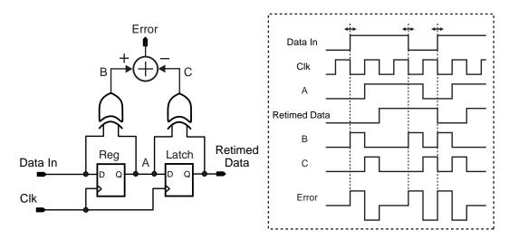
Figure A.7 A linear phase detector (Hogge topology).
