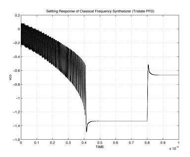
Figure A.3 Simulation plot for classical synthesizer (Tristate PFD).
