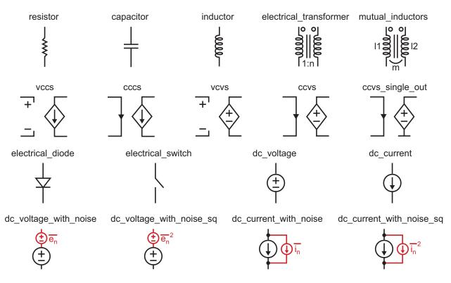
Figure 6.1 Electrical elements available in CppSim.
