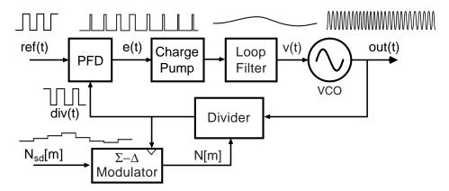
Figure A.4 A  $\Sigma$ - $\Delta$  frequency synthesizer.
