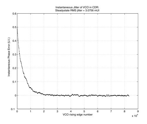
Figure A.8 Simulation plot for CDR (linear phase detector).
