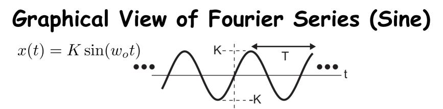
• We can plot Fourier coefficients as a function of index or frequency n
